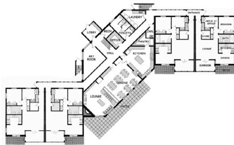
Image 8-11. Co-housing complex with central communal area between private dwelling units 8
